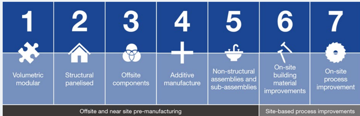
Figure 2.1: Offsite and Near-Site Pre-Manufacturing and Site-Based Building Processes
